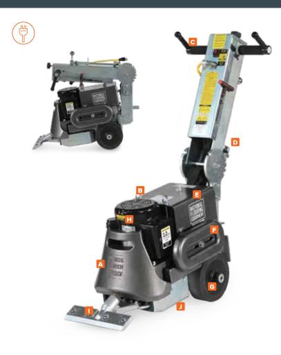
The Gladiator removes the worst of today's hard and soft goods, such as ceramic tile, wood floors, thin-set, sheet vinyl, linoleum, and more. Its compact design makes it ideal for use in confined spaces, while the side slide weights add extra head pressure when forward and improved traction when moved over the back wheels.
